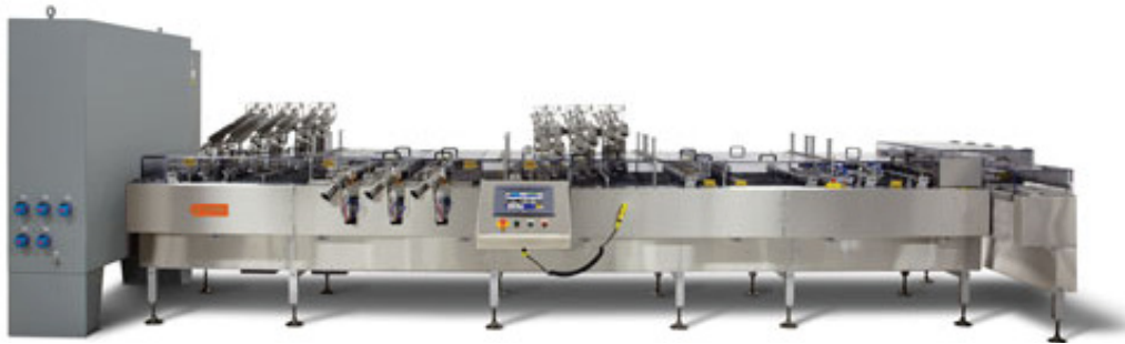
PT2-3 Sandwicking Machine shown with optional QS2 Row Combiner/Diverter
